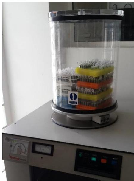
**Figure 2.** Lyophilization of plant material
