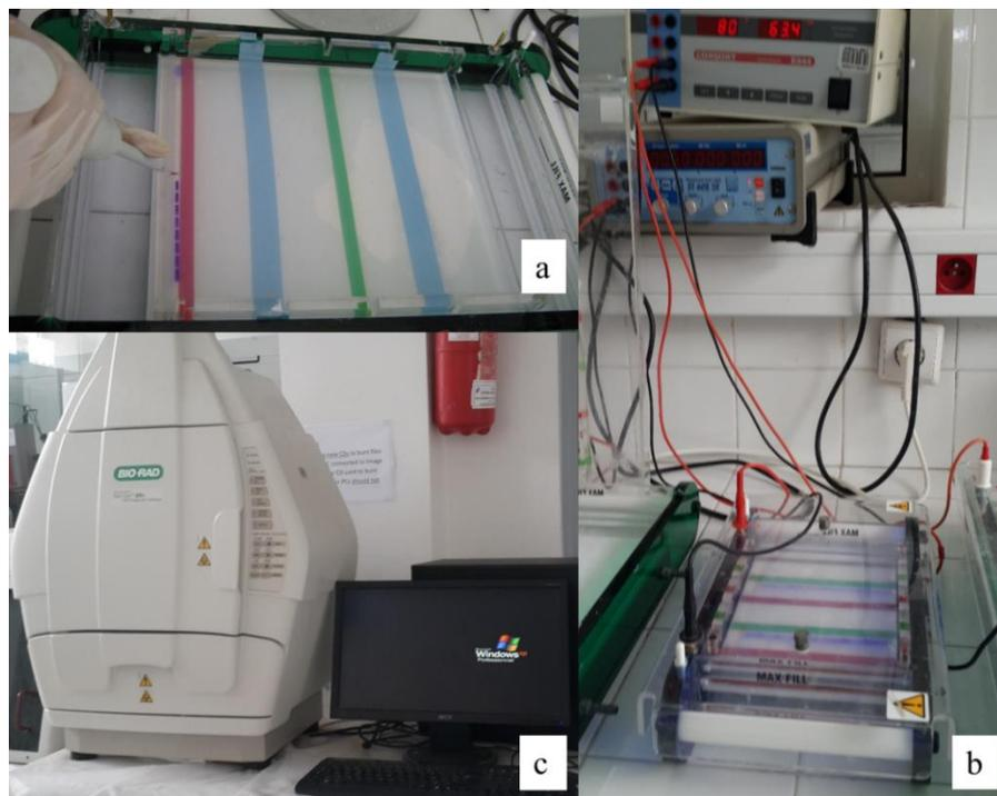
**Figure 6.** Deposit phase, running and visualization of 1% agarose gel
