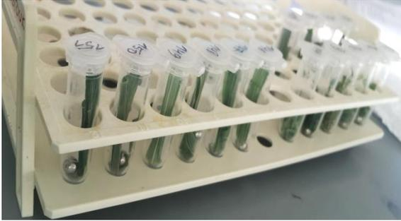
**Figure 3.** Steel beads are introduced at the bottom of each tube containing lyophilized material
