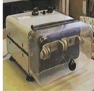
**Figure 4.** The lyophilized material is reduced to a powder using a Mechanical grinder
