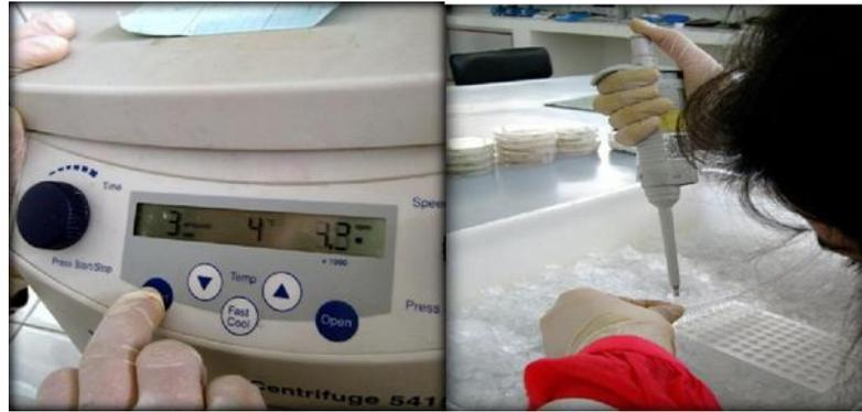
**Figure 8.** On the left, the master mix is being centrifuged and on the right 9  $\mu$ L of the mix are deposited in each PCR tube
